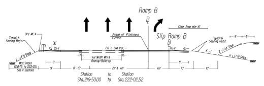
X Transition shoulder slope from match proposed pavement to -5% (Std GS-II) from sta.218-25 to sta.218-50.83
