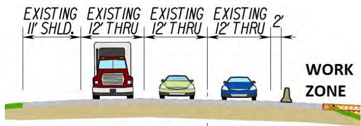
Figure 4.5.2.1 - Maintenance of full existing lane widths and full right shoulder on southbound I-95 during Stage 1 median work.
