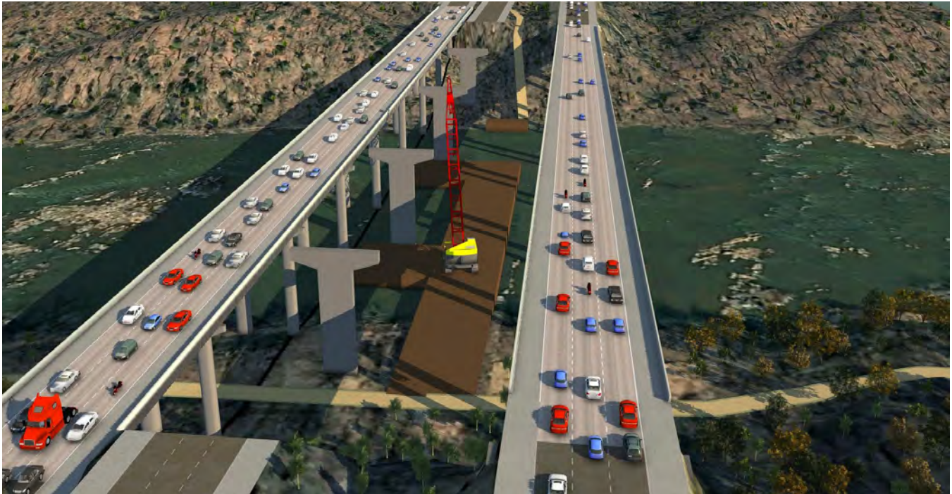
Figure 4.5.1.4 - Causeway with Open Channels at All Times
