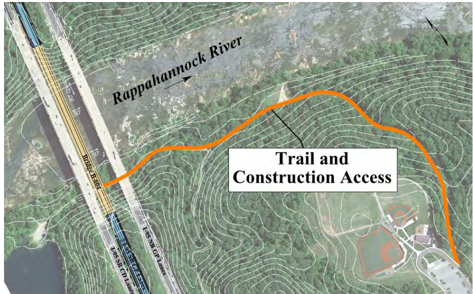
Figure 4.3.1.5 - Construction Access utilizing Quarry Road Through City-Owned Recreational Lands
