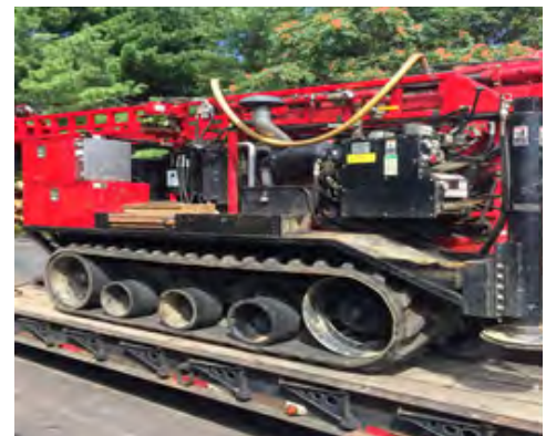
Figure 4.4.3.4 - Dietrich D-50 Track Rig
