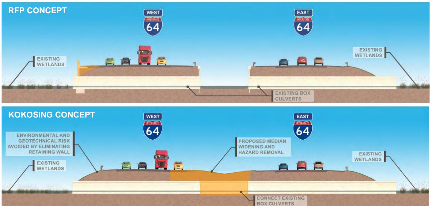
Figure 4.3.1-1: RFP Concept (top) and Kokosing Concept (bottom) at existing Quad Box Culvert at Sta 998+00
