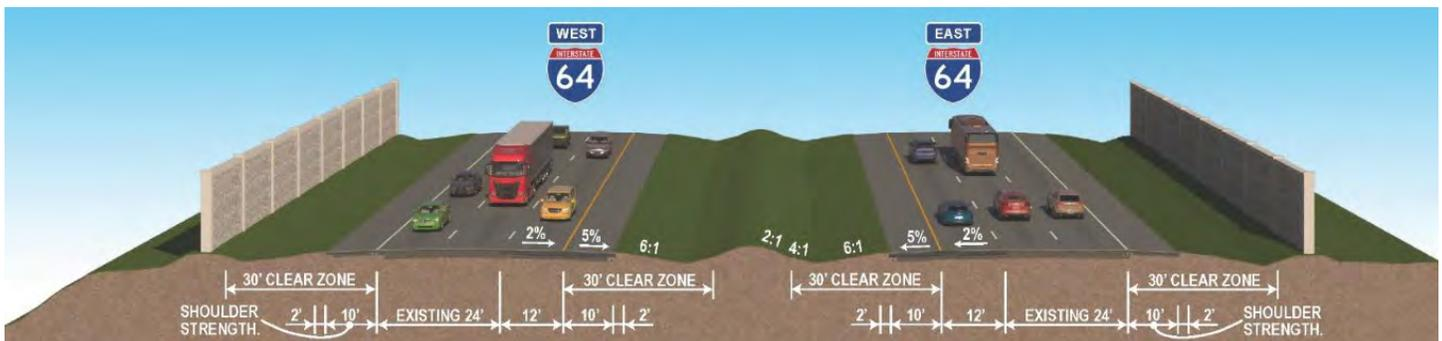
Figure 4.3.1-3: Proposed Roadway Typical Section
