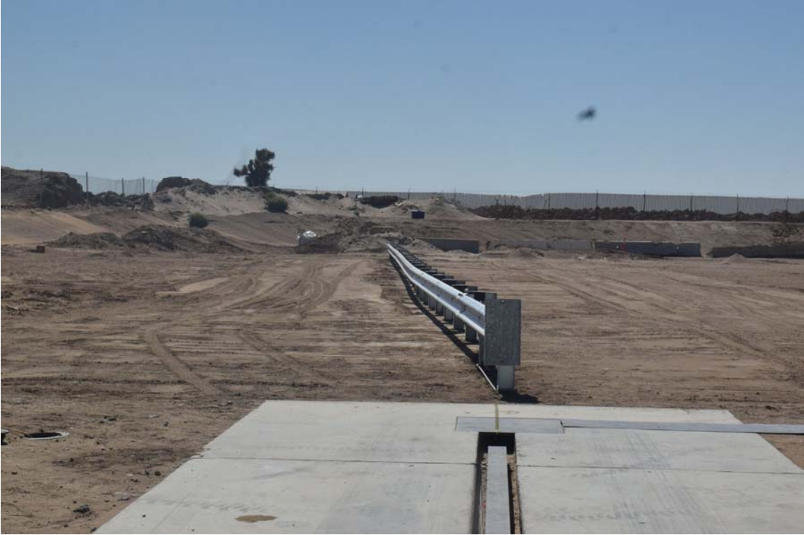
FIGURE 17. Pre-Test Front View of Test Article
