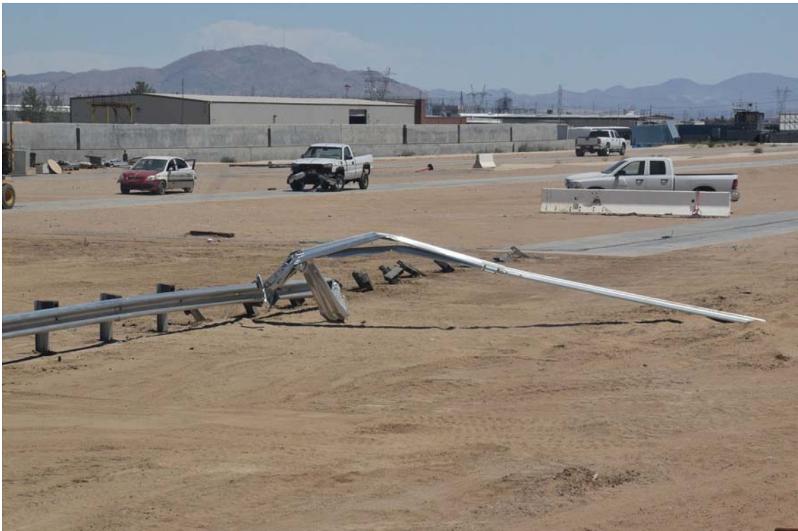
FIGURE 24. Post-Test Right Rear \frac{3}{4} View of Test Article
