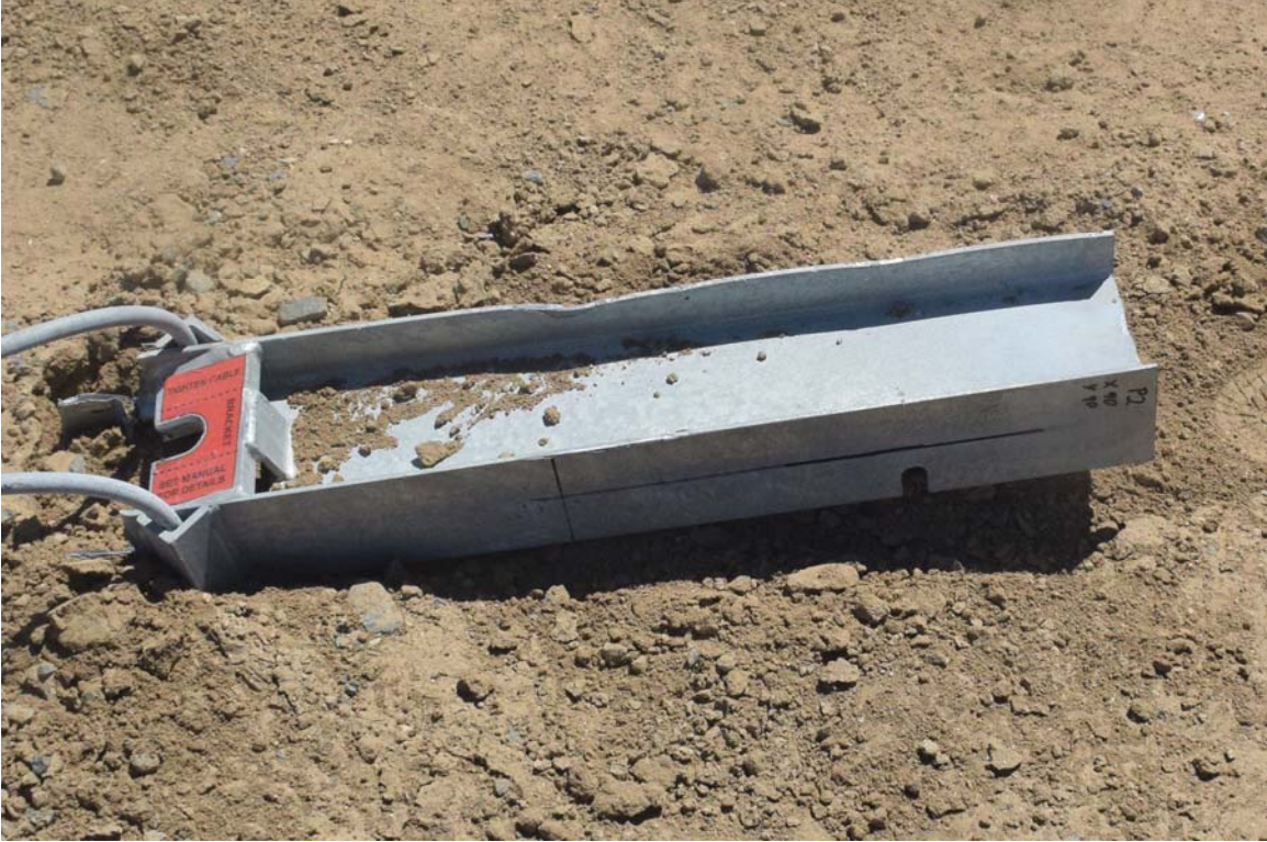
FIGURE 35. Test Article Damage
