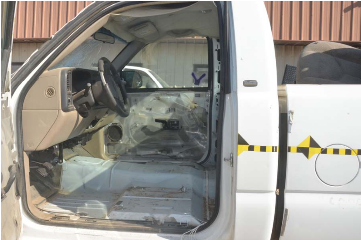
FIGURE 52. Post-Test Driver Side Occupant Compartment
