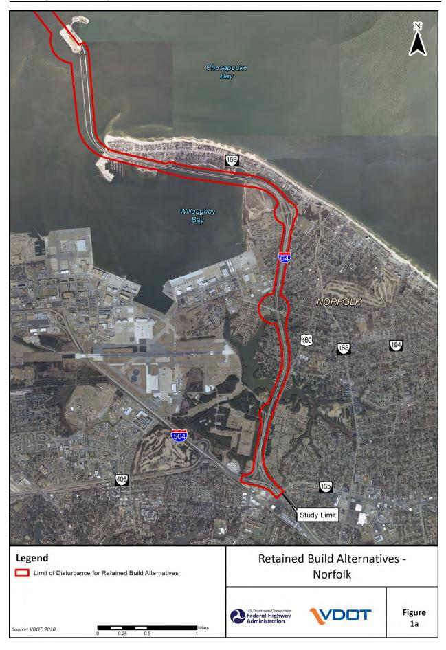
Interchanges within the corridor would be modified to accommodate the widened mainline section. Some interchanges would require elimination, reconstruction, realignment and/or lengthening of ramps, or similar modifications to surface streets, to meet geometric requirements per the American Association of State Highway and Transportation Officials (AASHTO) design criteria.
