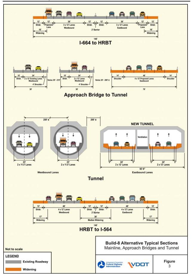
The existing approach bridges and tunnels would be rehabilitated, as described in Section 5.C. The alternative would include a new four-lane bridge-tunnel at the Hampton Roads crossing. Additional details of the new approach bridges and tunnel are provided in Sections 9.E and 9.F.
