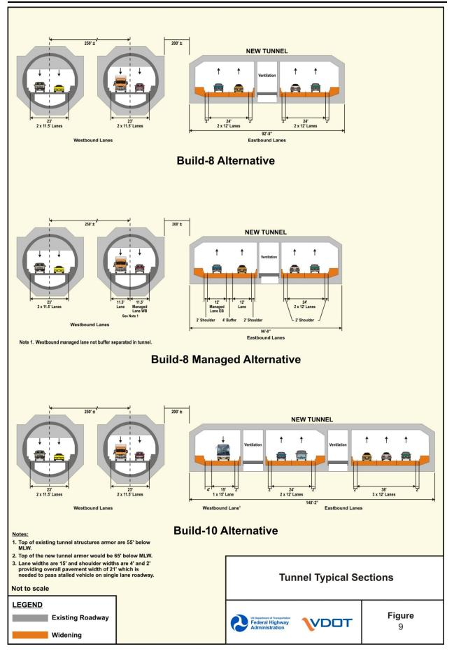
The existing river bottom would be dredged to provide a trench for the immersed tunnel. The existing tunnels would be protected during the widening of the islands and dredging operations for the new tunnel. Once the new tube sections were placed, the trench would be backfilled with aggregate and riprap of sufficient depth to protect the new tunnel from scour, normal channel dredging operations, and impacts from passing ships.
