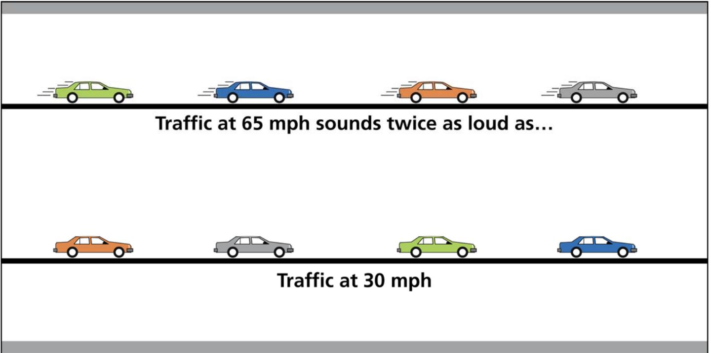
Figure 6: Effect of traffic speed on noise levels
