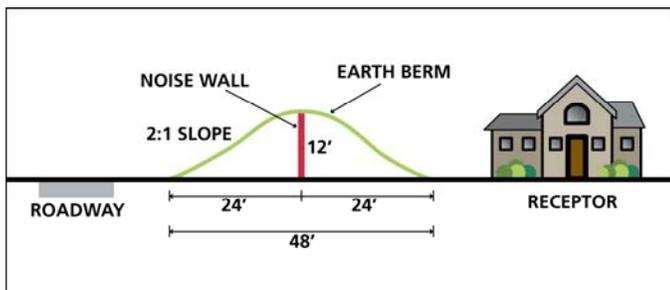
**Figure 14: Berm vs. Wall**
