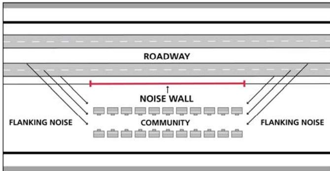
**Figure 11: Flanking Noise**
