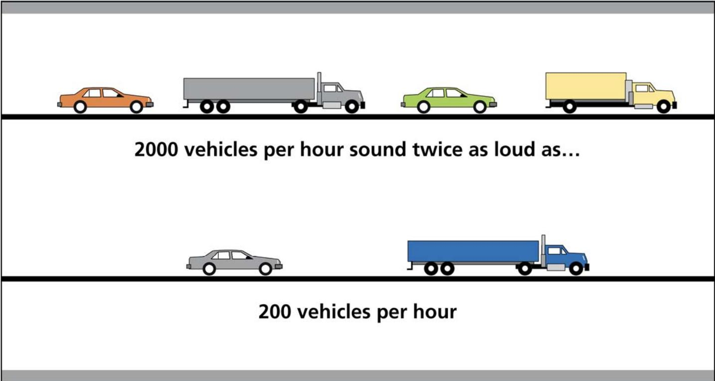
Figure 4: Effect of traffic volume on noise levels
