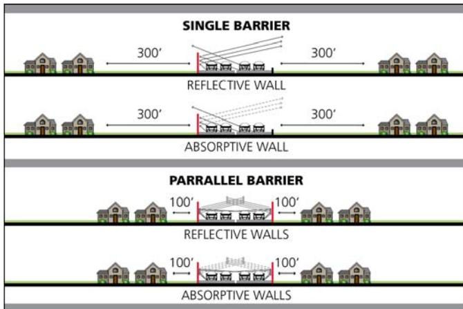
**Figure 8: Reflective/Absorptive walls**
