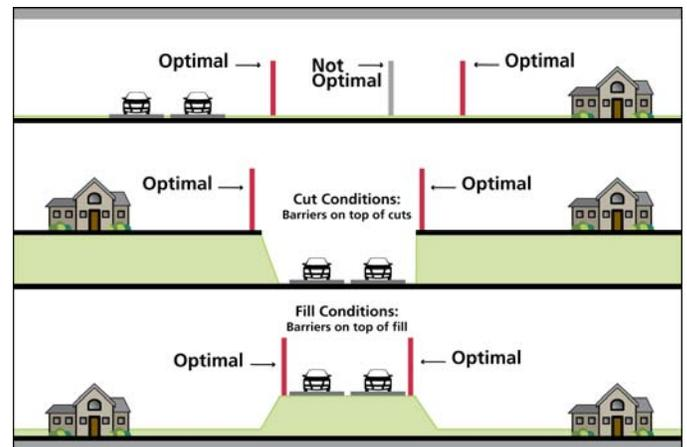
**Figure 10: Barrier placement**
