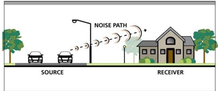
**Figure 7: Source-path-receiver concept**
