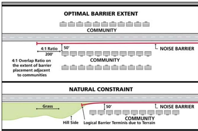
**Figure 12: Barrier design, minimizing flanking noise**
