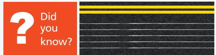
Brine is a mix of 23% salt and 77% water. It is sprayed as a liquid that dries to create white "brine lines" on the pavement.
